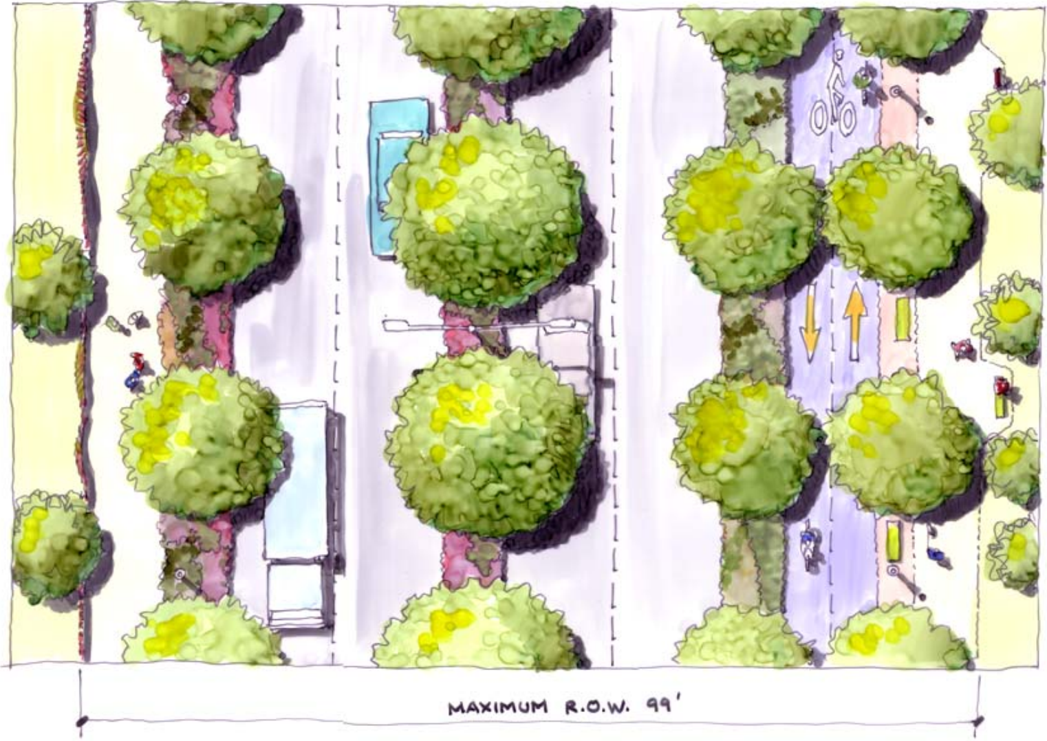
Typical Plan View - Condition A: Cargo Way Maximum R.O.W. Width 99' Cargo Way Conceptual Streetscape Plan
