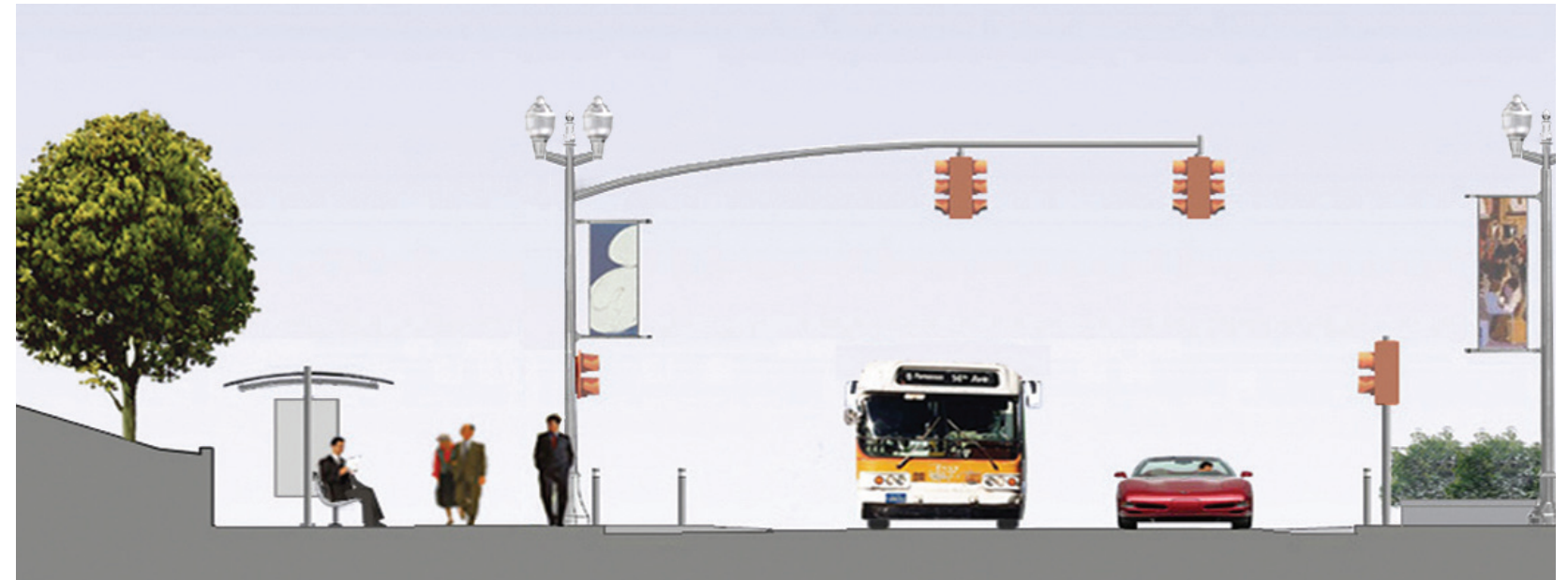
Figure 63. Sample light fixture coordination with MUNI catenary or traffic signal mast arm on Galvez Avenue
